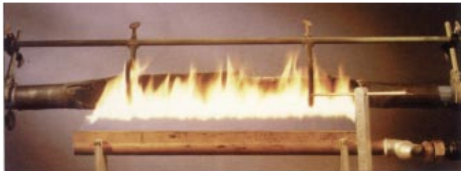
Photo 5: A fire-resistant Raychem joint maintaining its electrical integrity for more than 180 min. during a fire test according to IEC 331.
