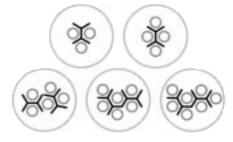
For each clip used, subtract 5 mm from the maximum cable diameter shown in the table to determine the maximum cable bundle diameter.
