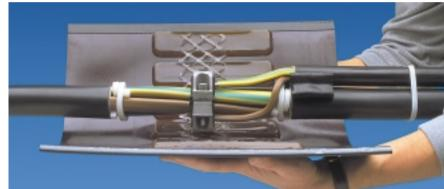
When closed, the wraparound overlaps the oversheath of the main and branch cables. The shrinking process is begun at the outer edges and continued towards the centre of the joint.
